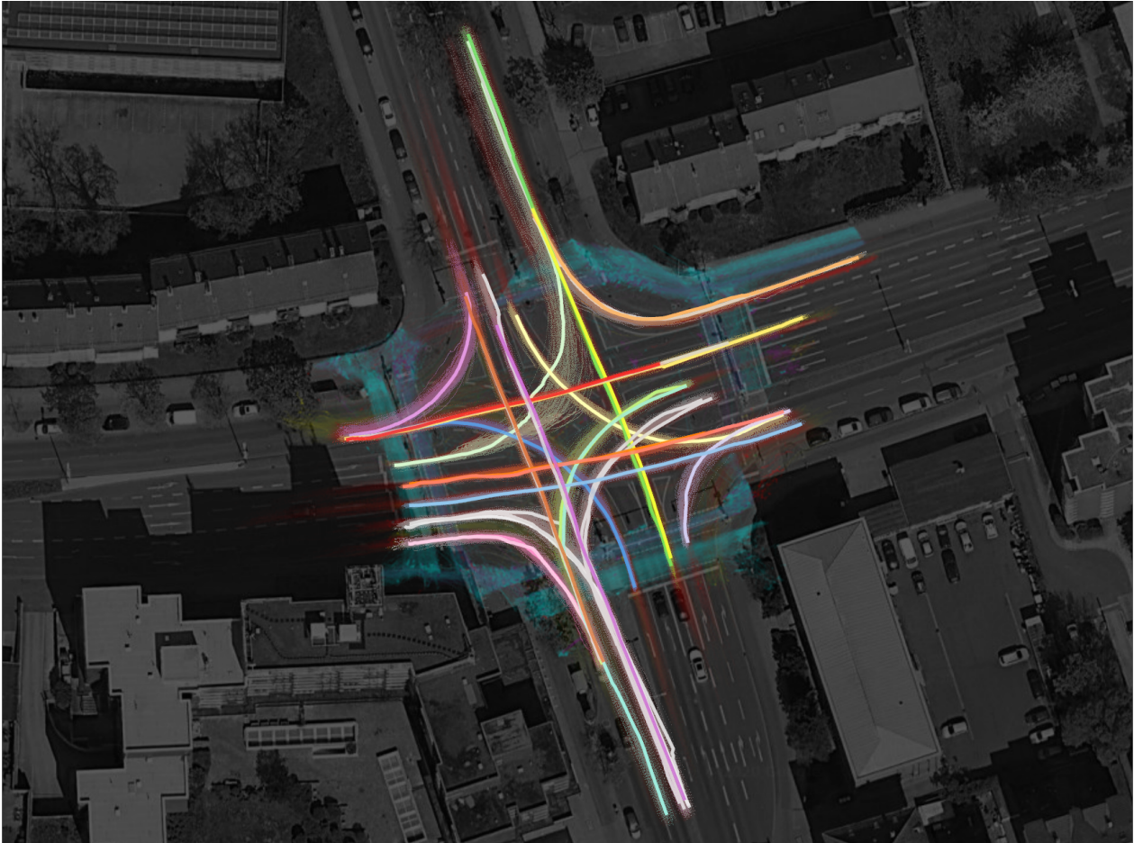
Trajectories of passenger cars, vans and trucks have been classified into their lanes (different colors) at an intersection in Lower Saxony, Germany. This data were used to learn a model of human-driven vehicles.
