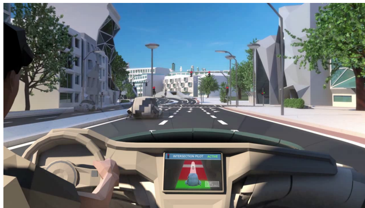
Figure 3: Driver's view when approaching a traffic-light. The driver-assistance system ensures an automated passage after the light switches to green without having to stop.
